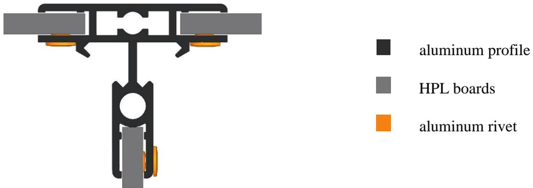
*Cross-section of the rear aluminium beam (T) in the locker S300*
