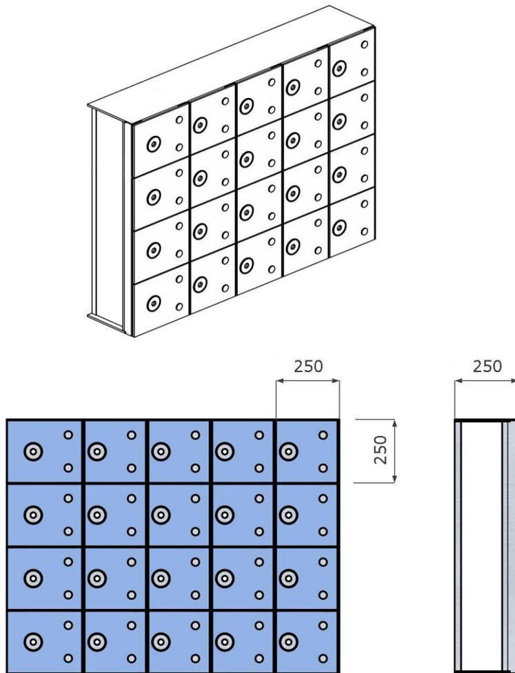
**Locker design:** the locker is designed with greater attention to safety and vandal-proof features, it is a modular structure (the lockers are installed side-by-side). The visible locker side can be terminated with HPL board or glass with various motifs, e.g. a promotion banner. The framework of locker is made of anodised aluminium.
