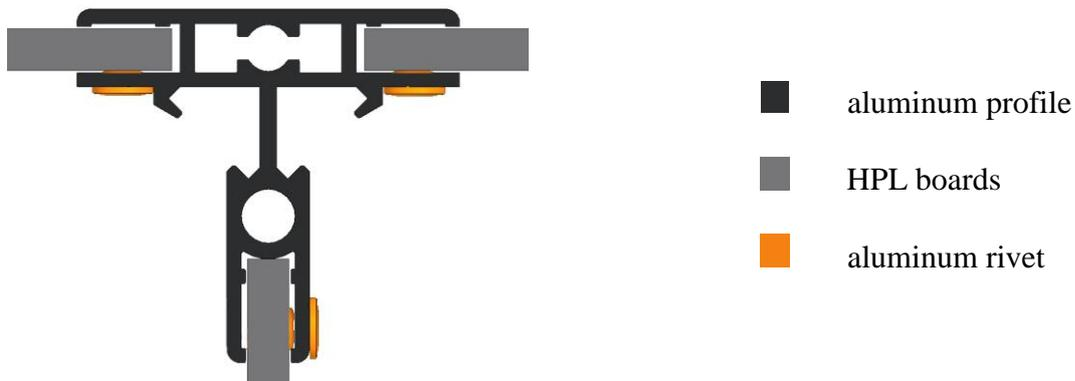
*Cross-section of the rear aluminium beam (T) in the locker S113*
