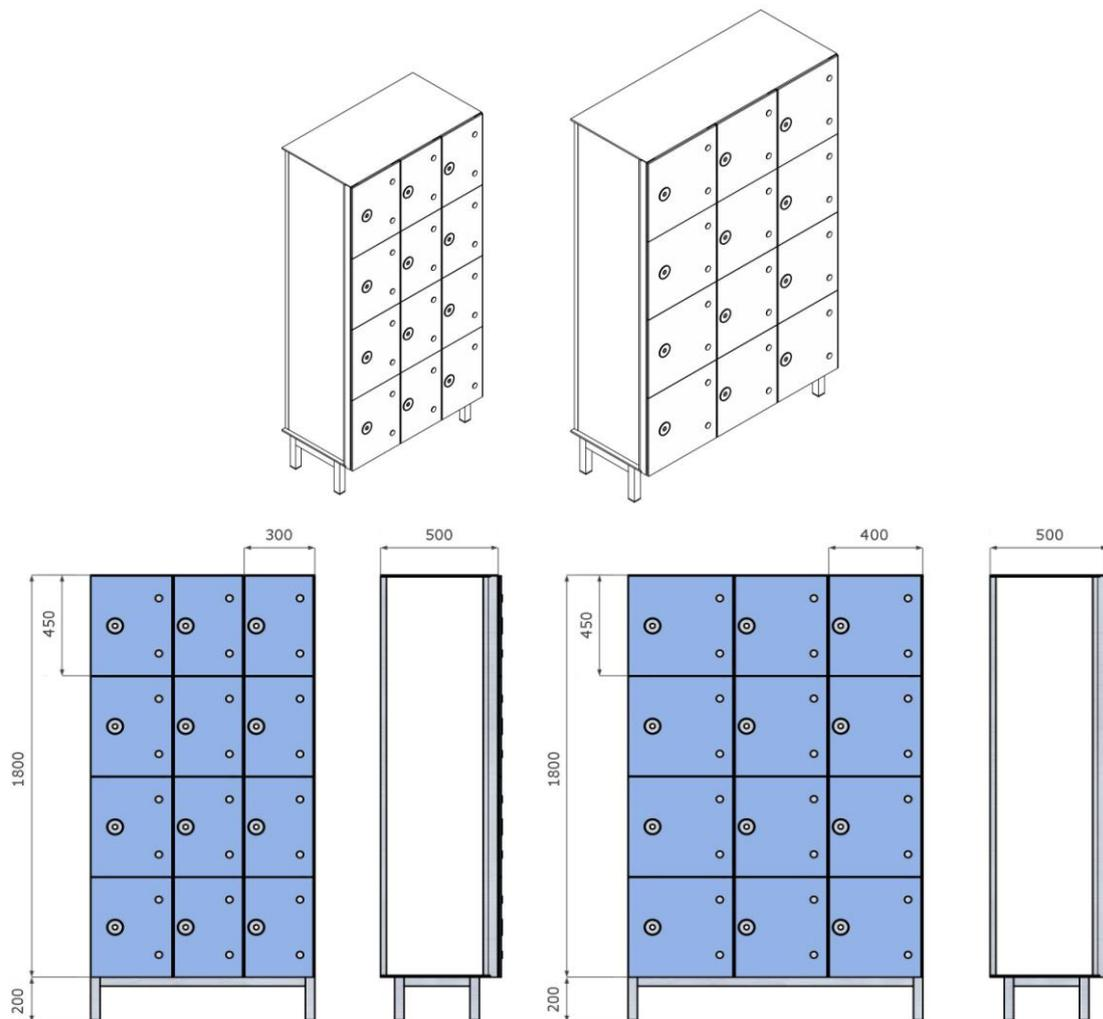
**Locker design:** the locker is split into four equal compartments and designed with greater attention to safety and vandal-proof features, it is a modular structure (the lockers are installed side-by-side). The visible locker side can be terminated with HPL board or glass with various motifs, e.g. a promotion banner. The framework of locker is made of anodised aluminium.
