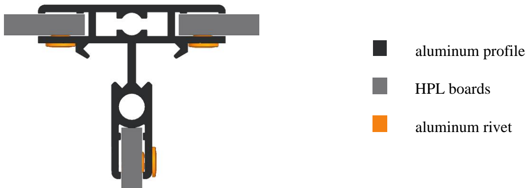
Cross-section of the rear aluminium beam (T) in the locker S103
