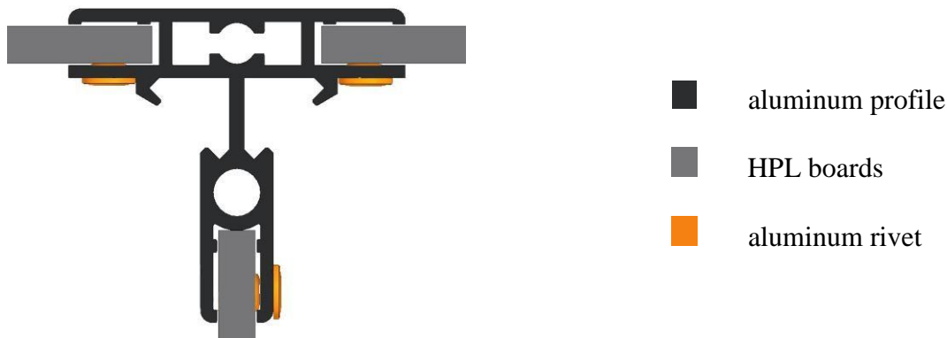
Cross-section of the rear aluminium beam (T) in the locker S103
