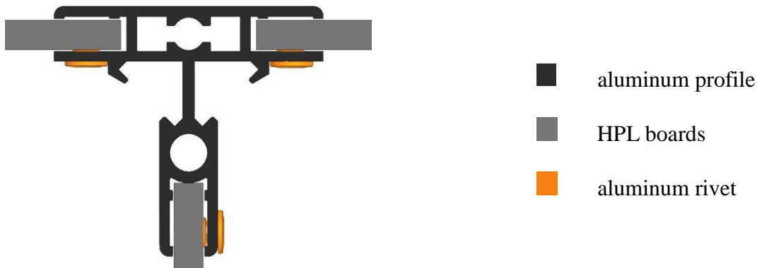
Cross-section of the rear aluminium beam (T) in the locker S102
