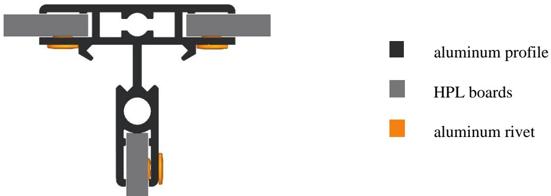
Cross-section of the rear aluminium beam (T) in the locker S102
